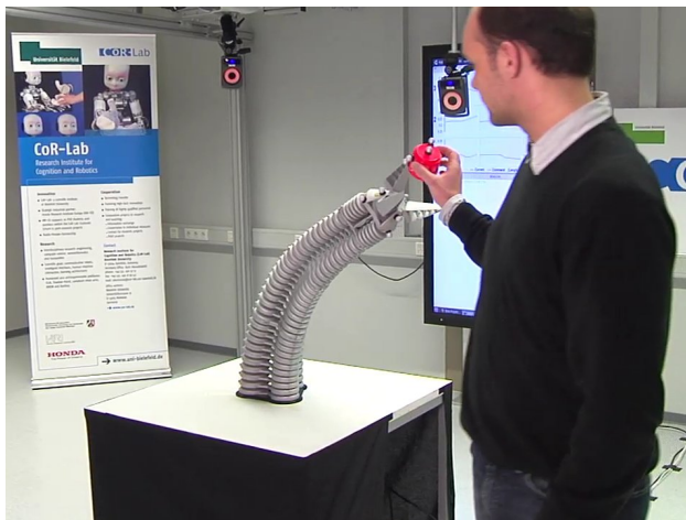
Fig. 3. Goal babbling allows to efficiently learn reaching with the Bionic Handling Assistant . The feedforward control with an inverse model allows to cope with intense sensory noise and delays.
