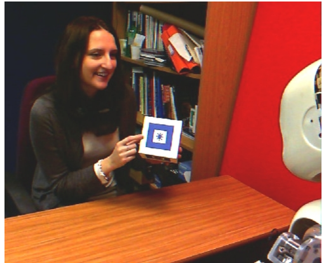
Fig. 1. One of the participants explaining shapes and colours to the iCub [9] robot. The shape explained is the blue sun inside of an ARToolKit [10] marker for the object detection.
